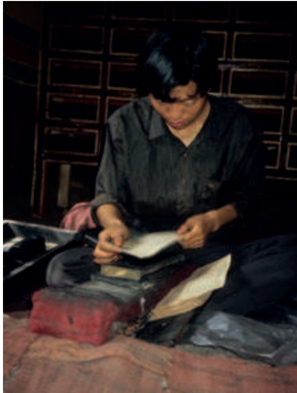
Applying paper to the inked block
