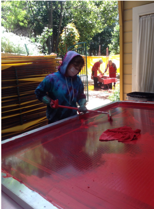
Left: Fig. 23 A volunteer cleans the silk-screen at the end of a printing run, using a squeegee to displace the tacky ink. Right: Fig. 24 A clean silk-screen screen dries in the foreground, while newly printed flags dry in the background. Photos taken by the author.
